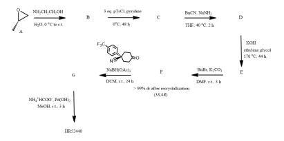
Figure 1: Route of synthesis for compound HR52440
